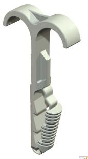
These push-fit clips are used when installing cables and pipes on walls and ceilings and when running flexible pipes on concrete and in the screed. The double push-fit clips can be used instead of nail clips in concrete and aerated concrete. The advantage of the push-fit clips is that they only have to be pushed into the drilled hole. Anchors and bolts are not needed.
