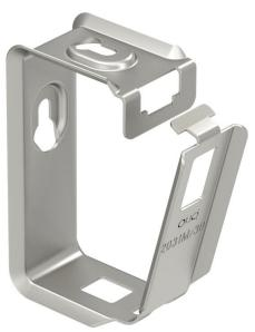
Metal grouped support for high mechanical stability, even in case of fire. Suitable for safe mounting above fire protection ceilings. Also approved as a cable-specific variant for the maintenance of electrical function to DIN 4102 Part 12. For wall and ceiling mounting. Lock can be opened without tools. Detailed information on the approved routing variants can be found in the appropriate testing documentation.
