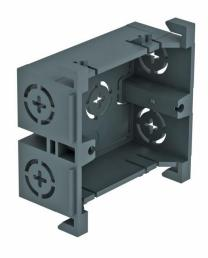
Front-locking, single device installation socket for British Standard switch systems. Insertion opening for cable diameters of max. 17 mm. Can be used in all device installation trunking of the Rapid 80 series and ISS service poles with 76.5 mm system opening.
