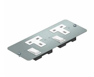
Cover plate with two switched single sockets for installation in mounting supports beneath GES service outlets and cassettes. Sockets with increased contact protection with screw connection, 3-pole, 13 A, 250 V~, corresponds to BS 1363.
