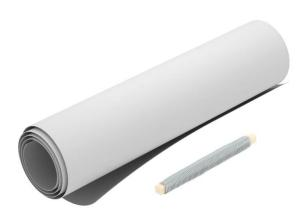
The fire protection bandage is used as cable insulation for individual cables, cable- and electrical installation pipe bundles (EIR). The insulation consists of a flexible bandage, fixed using wire. When surrounding the cables, take account of how often the appropriate medium must be surrounded. Refer to the approval for details. The bandage can be used directly next to Rockwool pipe insulation. Winding wire is included.
