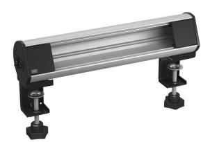
Ready-for-connection Deskbox DBL for the direct supply of workstations with power. With a Wieland GST18® connector and cable outlet at the left side of the profile. Toolless mounting with 2 fastening clamps for tabletop thicknesses of 8 to 40 mm and 40 to 70 mm. The Deskbox is not equipped and can be equipped with up to 5 installation devices of type Modul 45®.
