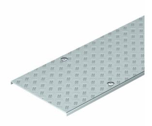
Cable tray cover for the walkable BKRS cable tray system. The basic cover is strip galvanised in a material thickness of 2 mm with additional aluminium chequer riveted on in a thickness of 4 mm, sturdy and non-slip. Turn buckle fastening with a turn buckle distance of 500 mm.
