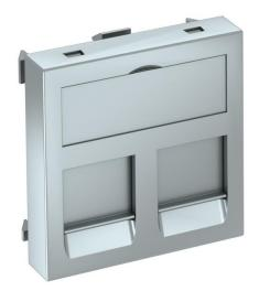
Data technology support with straight outlet and locking slider to accept two data technology connection modules with RJ45 socket. The locking fastening is suitable for horizontal and vertical installation in the system environment. Type C has a mounting opening of 19.30 x 14.80 mm and is designed for direct fastening of the data connection modules in the mounting opening.
