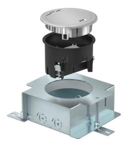
Round GES R2 service outlet with hinged cover, floor covering protection frame and UD GES R2 screed socket for installation in floors with screed structures in internal areas. Installation unit with a double power socket with a 33° insertion direction. At the side, next to the socket, there is space for an optional two connection sockets for data technology applications. When closed, the installation unit can be wet-cleaned. The minimum installation depth is 85 mm. Chrome-plated surface.
