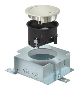
Round GES R2 service outlet with hinged cover, floor covering protection frame and UD GES R2 screed socket for installation in floors with screed structures in internal areas. Installation unit with a double power socket with a 33° insertion direction. At the side, next to the socket, there is space for an optional two connection sockets for data technology applications. When closed, the installation unit can be wet-cleaned. The minimum installation depth is 85 mm. Surface: Nickel-plated.
