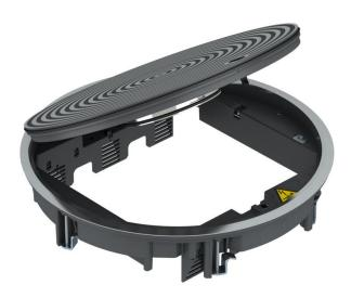
Service outlet with tube body for wet-cleaned floors for up to 12 individual Modul 45 devices in 3 UT4 universal supports, use in duct and trunking systems and system floors indoors.
