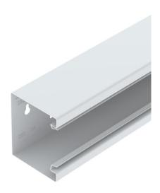
GS device installation trunking for mounting on the wall or on fastening panels. The GS device installation trunking possesses self-contacting locking straps to accept a sheet steel partition. The equipotential bonding between the trunking bases takes place using the trunking coupling. The protective measure and the equipotential bonding is guaranteed between the cover and the base by the self-contacting trunking cover. The real system opening is 76.5 mm. The cover must be ordered separately.
