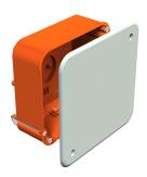
Cavity wall connection box for use in cavity walls with an installation depth of at least 50 mm and a plate thickness of 7-35 mm. With white cover and cover screws. Suitable for installation of standard rails (hat and support rails) for series terminals.
