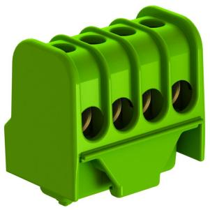
Protective conductor connection terminal strip, brass, steel screws, electrogalvanised and transparently passivated, nominal cross-section  $6 \div 16 \text{ mm}^2$ , nominal voltage 400 V, 1-pole, with terminal sockets, max. connectable conductors per terminal 4 x 16 mm<sup>2</sup>, 4 x 10 mm<sup>2</sup>, 8 x 6 mm<sup>2</sup> or 12 x 4 mm<sup>2</sup>.
