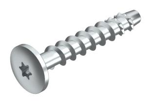
Bolt tie for direct mounting without additional anchors in cracked and uncracked concrete and masonry. With large round head to fasten mounting and profile rails. Torx drive T30.
