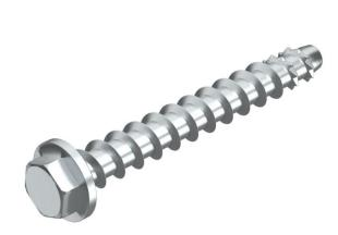
Bolt tie for direct mounting without additional anchors in cracked and uncracked concrete and masonry. With hex head drive and pressed washer to accept large loads. Suitable for fastening suspended loads from suspended supports and wall brackets.
