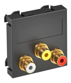
Multimedia support with three cinch connection sockets for audio-video, straight cable outlet, with labelling panel, three cinch sockets (RCA) with soldered connection, colour coding yellow / red / white. Support plate with locking fastening, suitable for horizontal and vertical installation in the system environment.
