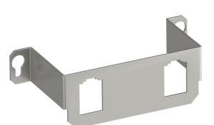
Mounting support to accept two data connection modules of the following types BTR: E-DAT; Dätwyler: MS and MS-N; Kerpen: VarioKeystone. Dimensions of a mounting opening in mm: 19.35/21.55 x 14.85. Suitable for GE2 installation unit with floor covering recess.
