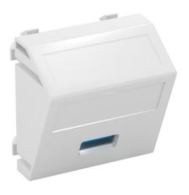
Multimedia support with one USB 3.0 connection socket, slanting cable outlet, with labelling panel, USB 3.0 type A socket with screw connection. Support plate with locking fastening, suitable for horizontal and vertical installation in the system environment.
