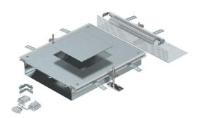
Ready-to-mount trunking extension unit with a device installation lid for the installation of an installation unit of nominal size 4, consisting of the trunking base (floor trough with side and floor covering guide profiles), trunking lid with blank mounting opening and a flushfloor end cover. The scope of delivery contains three height-adjustable wall fixing brackets, three screed anchors and trunking connection brackets.
