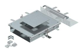
Ready-to-mount trunking extension unit with a device installation lid for the installation of a flush-mount unit of nominal size 9, consisting of the trunking base (floor trough with side and floor covering contact profiles), trunking lid with blank mounting opening and a flushfloor end cover. The scope of delivery contains 3 height-adjustable fixing brackets, 3 screed anchors, 1 lid butt support and 1 construction set for 90° angle
