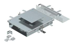
Ready-to-mount trunking extension unit with a device installation lid for the installation of a flush-mount unit of nominal size 6, consisting of the trunking base (floor trough with side and floor covering contact profiles), trunking lid with blank mounting opening and a flushfloor end cover. The scope of delivery contains 3 height-adjustable fixing brackets, 3 screed anchors, 1 lid butt support and 1 construction set for 90° angle
