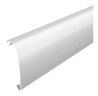
Trunking cover to create a design device installation trunking of the GAD series. "Soft" design version for complete coverage of the system opening and the switching and plug-in devices. The GAD OTA cover adapters are essential and must be planned on the trunking section with a max. spacing of 50 cm. A GAD OTD spacer must be placed between the trunking covers.
