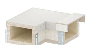
90° bend for PYROLINE® Con S El60 fire protection duct, type PLCS D061220, consisting of fibre glass light concrete which is resistant to water and frost for the creation of horizontal changes of direction of the duct. Mounted connectors ensure quick mounting in situ, whilst loosely placed covers ensure quick inspection and reassignment.
