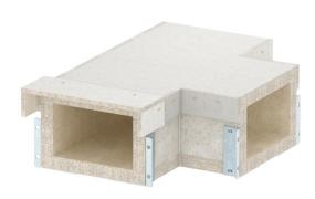
T piece for PYROLINE® Con S EI60 fire protection duct, type PLCS D061220, consisting of fibre glass light concrete which is resistant to water and frost, for the creation of T branches of the duct. Mounted connectors ensure quick mounting in situ, whilst loosely placed covers ensure quick inspection and reassignment.
