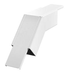
45° vertical bend, falling version, with intumescent fire protection mesh for PY-ROLINE® Rapid PLM installation duct. Suitable for direct wall and ceiling mounting, mounting below system floors and on support systems. Tool-free joint mounting with PLM SI joint connector. The cover is snapped on without tools, allowing rapid inspection and retroassignment. The cover overhang allows offset cover mounting for continuous equipotential bonding of the entire duct section.
