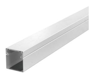
Metal installation duct with intumescent fire protection mesh for fireproof routing of cables. Classified as an installation duct El30, El60 and El90 according to EN 13501-2, tested according to EN 1366-5. The duct prevents the fire spread for the classified period of time, offering protection against the effects of a cable fire.
