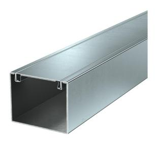
Metal installation duct with intumescent fire protection mesh for fireproof routing of cables. Classified as an installation duct El30, El60 and El90 according to EN 13501-2, tested according to EN 1366-5. The duct prevents the fire spread for the classified period of time, offering protection against the effects of a cable fire.
