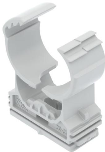
Highly stressable clip for accepting plastic or metal electrical and sanitary pipes as well as the electrical installation pipe Quick pipe. Universal fastening options on walls, ceilings and steel constructions, both indoors and outdoors. Flexible clamping range of several millimetres. Toolless pipe mounting. Connectable to each other to Ø 32 mm, also with the OBO Quick or Multi Quick clip. For variable distances and clip quantity mountable on a profile rail.
