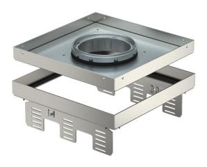
Height-adjustable cassette, decoupled from the floor, of nominal size 9, for tube bodies, for the installation of accessories in dry or wet-cleaned floors for indoor use, for mounting in underfloor boxes UZD250 or UZD350, either in conjunction with a mounting lid DUG../9 or in UGD250-3/9 or UGD350-3/9. Mounting takes place using height adjustment brackets (order separately) in the aluminium frame profile of the underfloor boxes.
