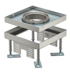
Height-adjustable heavy-duty cassette for tube bodies of nominal size 4 for the installation of devices in duct systems, raised and cavity floors in interior dry or wet-care floors. Load class 1 to 10 kN.
