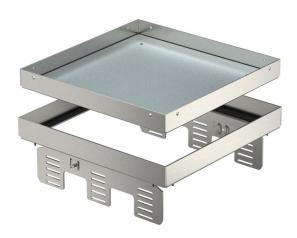
Height-adjustable "blank" cassette, decoupled from the floor, for the creation of an inspection opening of nominal size 9 in dry or wet-cleaned floors for indoor use, for mounting in underfloor boxes UZD250 or UZD350, either in conjunction with a blanking lid DUG../9 or in UGD250-3/9 or UGD350-3/9. Mounting takes place using levelling profiles (order separately) in the aluminium frame profile of the underfloor boxes. Only suitable for smooth floor coverings.
