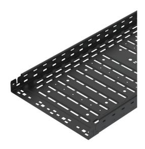
Cable tray with integrated quick-fastening system. Strip-galvanised surface, visible areas powder-coated in jet black (RAL 9005). Continuous side perforations of 7  $\times$  20 mm for the installation of additional connection and mounting components. With 11 mm perforation in the base for direct threaded rod suspension. Usable length 3,000 mm.
