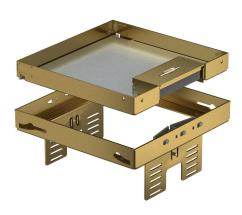
Height-adjustable cassette, decoupled from the floor, of nominal size 4, with cord outlet, for the installation of accessories in dry-cleaned floors indoors, for mounting in underfloor boxes UZD250 or UZD350, either in conjunction with a mounting cover DUG../4 or in UGD250-3/4 or UGD350-3/4. Mounting takes place using height-adjustment brackets (order separately) in the aluminium frame profile of the underfloor boxes.
