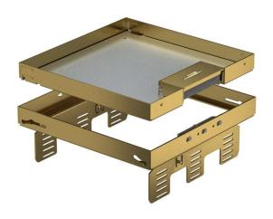
Height-adjustable cassette, decoupled from the floor, of nominal size 9, with cord outlet, for the installation of accessories in dry-cleaned floors for indoor use, for mounting in underfloor boxes UZD250 or UZD350, either in conjunction with a blanking lid DUG../9 or in UGD250-3/9 or UGD350-3/9. Mounting takes place using levelling profiles (order separately) in the aluminium frame profile of the underfloor boxes.
