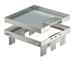
Height-adjustable cassette, decoupled from the floor, of nominal size 9, with cord outlet, for the installation of accessories in dry-cleaned floors indoors, for mounting in underfloor boxes UZD250 or UZD350, either in conjunction with a mounting cover DUG../9 or in UGD250-3/9 or UGD350-3/9. Mounting takes place using height-adjustment brackets (order separately) in the aluminium frame profile of the underfloor boxes.
