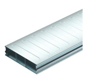
Underfloor trunking (2 piece) for routing cables in screed-covered underfloor systems, according to EN 50085-2-2. Removable and continuously lockable trunking cover. With separating retainers in the trunking base. Maximum load-bearing capacity to 1.5 kN. Only compatible with the UZD250-4/350-4
