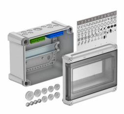
Distribution box with terminal strip for surface mounting, for the current sub-distribution in interior and protected exterior areas, in accordance with IEC 439-3. With pre-mounted 35 mm hat profile rail. IP66 protection type and IK07 protection rating. Transparent cover to screw on, with cut-out.
