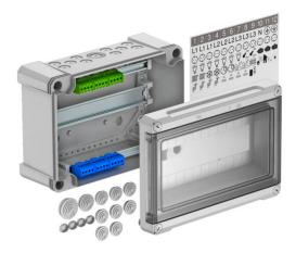
Distribution box with terminal strip for surface mounting, for the current sub-distribution in interior and protected exterior areas, in accordance with IEC 439-3. With pre-mounted 35 mm hat profile rail. IP66 protection type and IK07 protection rating. Transparent cover to screw on, with cut-out.
