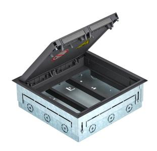
Square screed socket with GES9 UGE service outlet for use in screed floors for indoor use. With pre-marked insertion openings for pipelines (M20/M25) on all four sides
