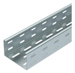
SKS 60 = heavy-duty cable tray system with 60 mm side height. The cable tray, type SKS, should also be used for the maintenance of electrical function. For additional data, please refer to BSS fire protection systems. Magnetic shield insulation without cover 20 dB, with cover 50 dB.
