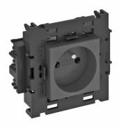
Earthing pin socket with connection to side, Single 0°, with increased touch protection, with screwless terminals, 2-pin, 16 A, 250 V $\sim$ , with connection terminals to IEC 60884-1, suitable for the installation in Rapid 80 device installation trunking systems.
