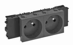
Earthing pin socket with connection to side, Double  $0^\circ$ , with increased touch protection, with screwless terminals, 2-pin, 16 A, 250 V~, with connection terminals to IEC 60884-1, suitable for the installation in Rapid 45 device installation trunking systems.
