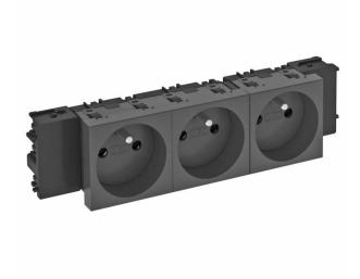
Earthing pin socket with connection to side, Triple  $0^\circ$ , with increased touch protection, with screwless terminals, 2-pin, 16 A, 250 V~, with connection terminals to IEC 60884-1, suitable for the installation in Rapid 45 device installation trunking systems.
