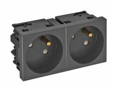
Socket with earthing pin and side connection, Double 33°, with increased touch protection, with screwless terminals, 2-pin, 16 A, 250 V~, with connection terminals to IEC 60884-1.
