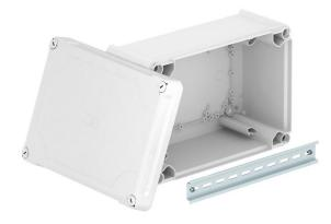
Closed junction box for the connection of cables and lines indoors and in protected outdoor areas. Rectangular design without entries. Suitable for wall and ceiling mounting, on mounting panels and threads in the floor. With the option to fasten inside and to mount via the corner domes. High, transparent cover with quick lock, sealable. Made from halogen-free and UV-resistant materials.
