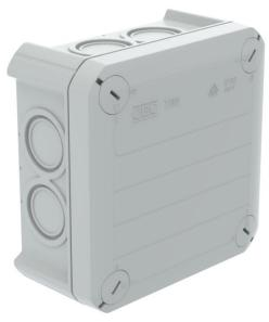
Junction box for the connection of cables and lines indoors and in protected outdoor areas. Square design with knock-out entries to the sides and knock-out entries in the bottom. Suitable for wall and ceiling mounting and on mounting panels. With the option to fasten inside and to mount via the corner domes. With fixed clamping cover. Made from halogen-free and UV-resistant materials.
