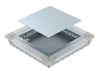
Underfloor accessory box with mounting lid and lid blanking plate with sheet steel side walls. For the installation of a square GES9 55 service outlet in screed heights of 55 mm or more. Height can be infinitely adjusted to the nominal screed height and the screed can be worked flush to the screed scraping edge. With 7 x M20, 3 x M25, 4 x M32 pipe insertion openings on each side. Usable pipe size at a system height of 55 mm: M20.
