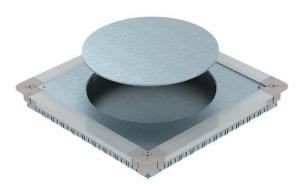
Underfloor accessory box with mounting lid and lid blanking plate with sheet steel side walls. For the installation of a square GES9 55 service outlet in screed heights of 55 mm or more. Height can be infinitely adjusted to the nominal screed height and the screed can be worked flush to the screed scraping edge. With 7 x M20, 3 x M25, 4 x M32 pipe insertion openings on each side. Usable pipe size at a system height of 55 mm: M20.
