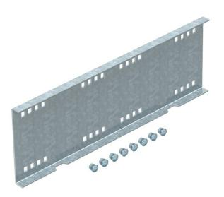
Straight connector for straight connections of cable trays, wide span cable trays and ladders with a side height of 160 mm. Including appropriate bolts, washers and nuts.
